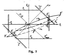
In case (1) the control synthesis is effected if the instant  $t_3$  and the instant  $t_5$  – the instant of crossing over to the trajectory segment with  $u = \pm u_0$ , passing through the origin (Fig. 3) – have been expressed in terms of the system's phase coordinates. The variation of the plant's phase state on the terminal segment is described, with due regard to (3, 2), by the following equations:
